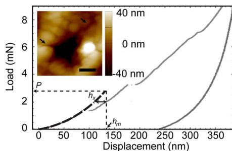
**Figure 1.** Indentation load-depth response, showing pop-ins and parameters  $h_x$ ,  $h_m$ , and  $P$  used to calculate fracture toughness  $K_{Ic}$ . Inset shows an atomic force microscopy (AFM) contact mode image of an individual indent exhibiting radial cracks highlighted by black arrows. The scale bar is 1  $\mu\text{m}$ .
